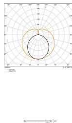
**Scheda tecnica Ledvance Tubo LED T8 EM Performance Conventional (EM), Mains (AC) Ultra Output 23.1W 3700lm - 840 Bianco Freddo | 150cm - Sostitutiva 58W**
